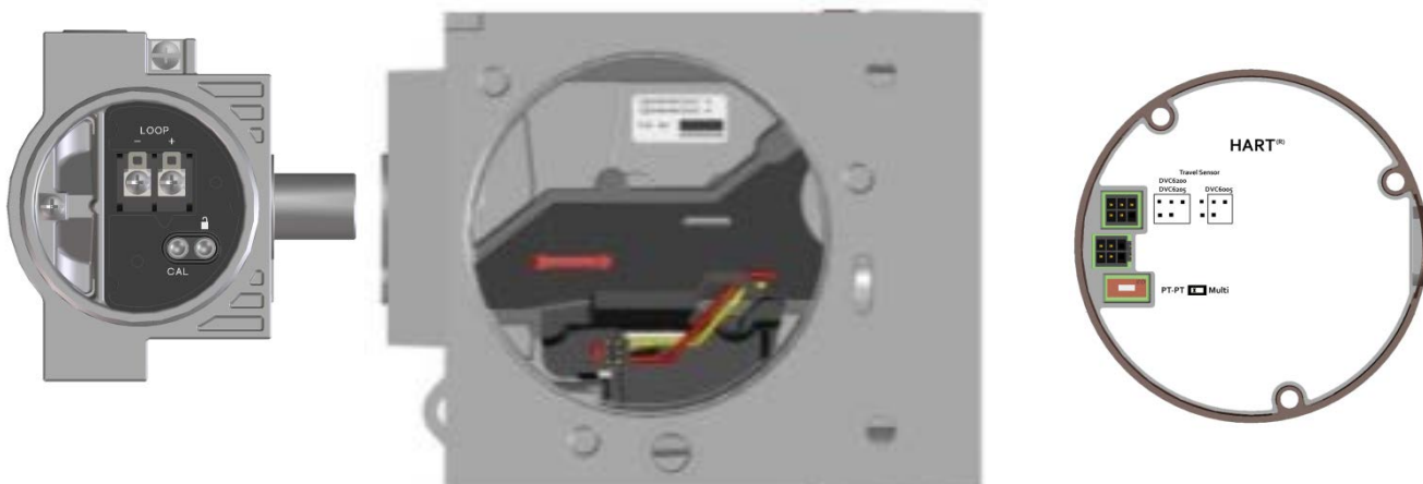
Figure 1. Images of new elements: Terminal Box, Rear Housing, and PWB (with new Firmware)
